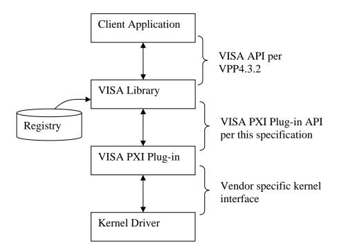
Figure 1 VISA PXI Plug-in mechanism provides standard access to vendor specific kernel drivers
