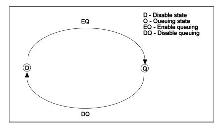
Figure 3.7.1 State Diagram for the Queuing Mechanism
