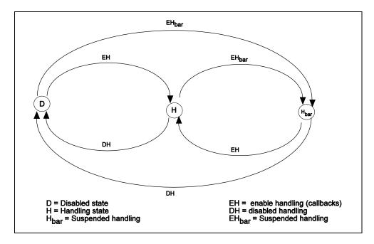
Figure 3.7.2 State Diagram for the Callback Mechanism
