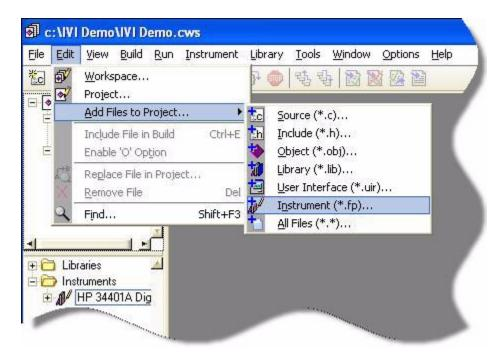
**Note**: Any of the three files listed above will work. Adding one of the HP 34401A instrument driver files loads that instrument driver. View the available functions in the library tree in the workspace window.
